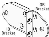
2. With the Universal Cord Tensioner (UCT) at the bottom of the bead chain loop, position it at the desired location.
