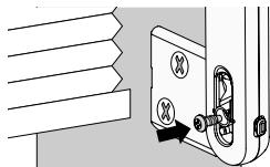
8. Ensure the bead chain can move freely through the UCT without engaging the lock. The center of the screw hole should be aligned with the notch in the UCT ( $\pm \frac{1}{8}$ ").
