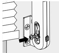
8. Ensure the bead chain can move freely through the UCT without engaging the lock. The center of the screw hole should be aligned with the notch in the UCT ( $\pm 1/8"$ ).
