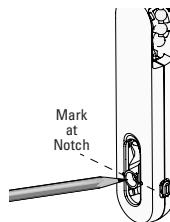
4. Hold the IB bracket with its center hole aligned with the mark and mark both hole locations.
