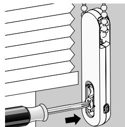
**CAUTION:** Do not overtighten the mounting screw. This can prevent the UCT from functioning properly and increase bead chain wear.
