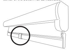
Wider shades have (2) Handles – to precisely determine the correct position for each handle, divide the total width of the shade by 4, and then attach one handle that distance from each outside edge of the bottom rail – always grasp both handles when lifting and lowering the shade.
