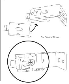
To adjust head rail extension, remove the shade from the mounting brackets by pressing on the plastic tabs at the front of each bracket. Then loosen the nut and bolt, and move the mounting brackets forward or backward as preferred.
