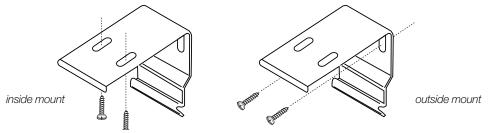
Attach each bracket to the inner top of the window opening using the screws provided. Pre-drill the screw holes using a 5/64" drill bit.
