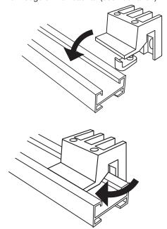
Position the tongue on each bracket so that it engages the slot in the head rail – tighten with a screw driver. Check carefully to assure that each bracket is properly secured.
