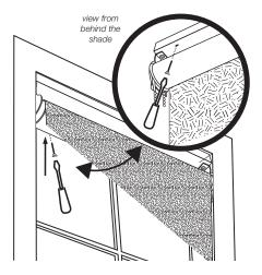
the front edge of the window opening (or position as desired), making sure that the shade is centered in the window opening – then push up on the screws so that the screw heads leave tiny impressions in the top of the window frame. Now, use the impressions as a guide and pre-drill the mounting holes using a 5/64" drill bit – then screw the shade in place.
