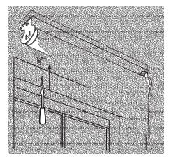
Place the head rail against the brackets as illustrated – center the shade over the window opening – then mark the location of each mounting hole on the head rail. Pierce the fabric at the hole locations using the tip of a screw, then pre-drill the mounting holes using a 5%4" drill bit. Attach the shade to the brackets using the 3¼" screws provided.
