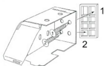
Align holes in back of bracket to holes in spacer block and secure to wall with screws. Two spacer blocks per bracket may be used for additional projection.
