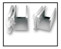
*Valance Installation Cont.* - To attach provided clips to the front of the headrail, twist Hidden Clip or push down on C-Clip to snap in place. Install one bracket at each end of the headrail and space others evenly. Do not place clips more than 48" apart.
