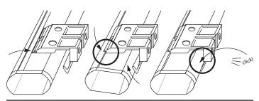
Lift the head rail into position such that the inner front edge of the head rail slides into the slot at the front of each bracket. Push the head rail upward until the flexible tab at the bottom of each bracket snaps onto the back of the head rail. Check carefully to assure that each bracket is properly secured.
