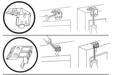
**Step 4.** Attach Handle(s) [Applies to cordless shades only] Attach the Handle to the bottom rail as illustrated. The handle is designed to minimize contact with the shade fabric.
