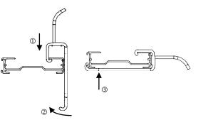
To install the handle, place handle to bottom rail. Flip over and snap into the groove of the rail.
