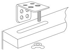
desired and center it over the window opening - mark the exact location of each bracket with a pencil. Remove the brackets from the head rail and position each bracket at the marked location. Mark the location of each screw hole with a pencil.
