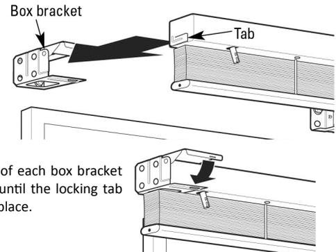
Lower the front gate of each box bracket and press until the locking tab clicks into place.
